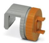
The optional holding device ensures the Rogowski coil is securely seated on busbars that are 5 ... 10 mm thick. During installation, the coil housing is pushed onto the flange of the holding device and snaps in automatically.
