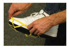
3) Extend positioning straps (D) around heel of shoe.
