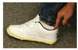
5) Test each foot grounder on an ESD footwear tester to confirm proper installation.
