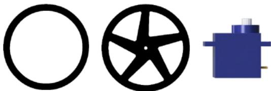
**STEP 1:** Stretch the O-Ring round the wheel, this will act as a tyre for :MOVE mini. Press fit the wheel onto the servo shaft and repeat for the opposite side.
