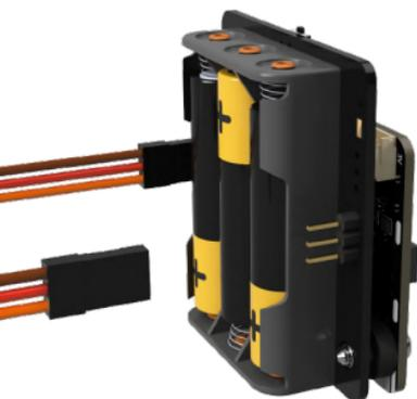
**STEP 1:** Plug the servo cables back into the Servo:Lite board. The left servo should plug into the left-hand side of the board and vice versa. The cables should be threaded down the gaps on either side as shown below.
