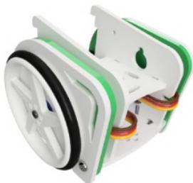
**STEP 2:** Clip the Servo:Lite board under the hooks on the inner side plates and slide it between the outer plates.
