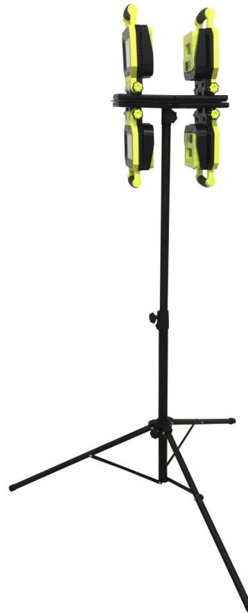
The TRIPOD-360 is a solid tripod that can hold up to 4 Unilite site lights at once, with 2 being placed on the top and 2 underneath. It can be dropped to 960 mm or raised to 1930 mm via the ergonomic grips.
