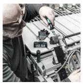
Many screws particularly in assembly and maintenance applications – have to be tightened with controlled torque to ensure the dependability of the screw connection and/or to avoid damage to the screw or work piece. Wera's adjustable torque screwdrivers are the ideal tool for this. They feature a torque range of 0.3 Nm to 8.8 Nm, two different handles, measurement accuracy of ± 6 % and Rapidaptor technology for rapid bit change.
