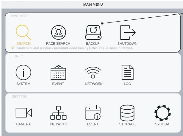
**OPERATE: BACKUP:** Plan backup of recorded video, to external media (External HDD or USB memory).
