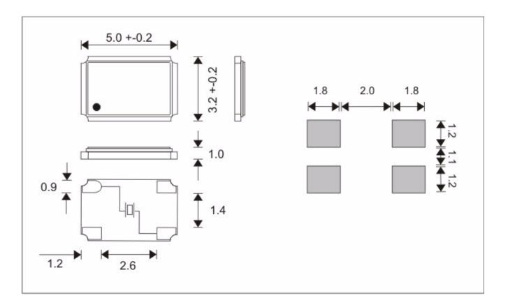
Holder Style Mode Adjustment Tolerance Temperature Stability Operating Temp. Range Load Capacitance ESR Static Capacitance (C0) Ageing Marking 5x32x1 4-Pad Fundamental ± 30PPM at 25°C ± 30 PPM -40°C to +85°C 18 pF 50 Max Ohm Unspecified pF +/-5ppm 1st Year Max AEL10.000 ww/yy
