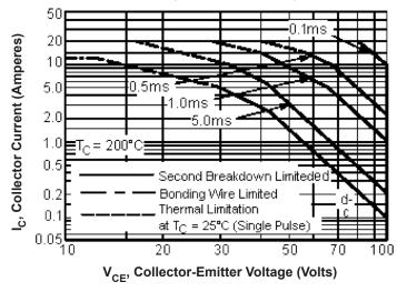
Newark.com/multicomp-pro Farnell.com/multicomp-pro Element14.com/multicomp-pro There are two limitations on the power handling ability of a transistor: average junction temperature and second breakdown. Safe operating area curves indicate  $I_C - V_{CE}$  limits of the transistor that must be observed for reliable operation; i.e., the transistor must not be subjected to greater dissipation than the curves indicate.
