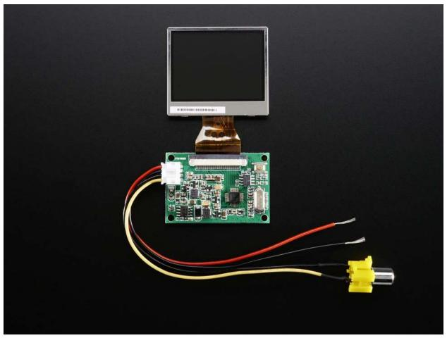
To demonstrate it, we took some photos with the display connected to a Raspberry Pi, but it will also work connected to any analog composite-video
