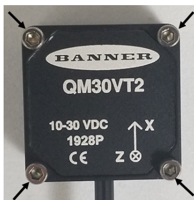
Figure 7. QM30VT2 mounted to the BWA-BK-014 bracket
