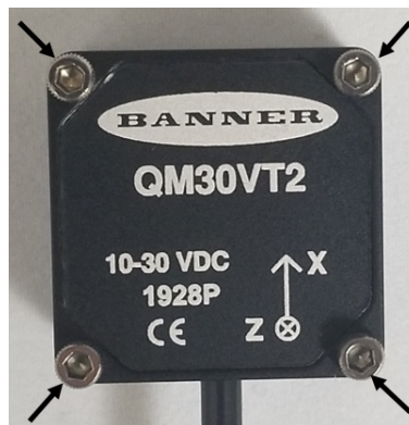
Figure 10. QM30VT2 mounted to the BWA-BK-013 bracket
