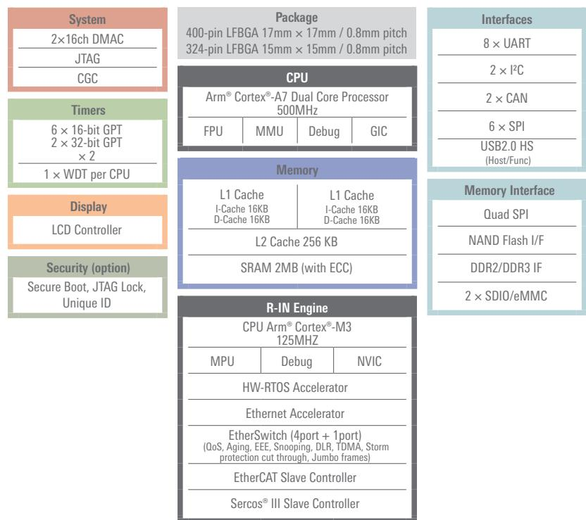
■ Application example: Programmable logic controller Block diagram
