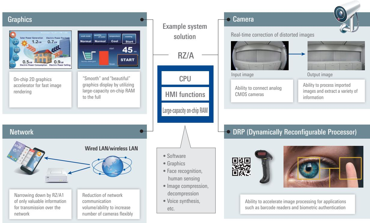
With ample peripheral functions and software, a single chip can cover a wide range of fields, including display, camera input, communication, and audio functions.
