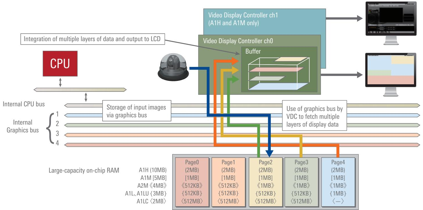
The bus configuration with independent buses for images and hardware-based superimposition processing make it easy to create graphical applications.
