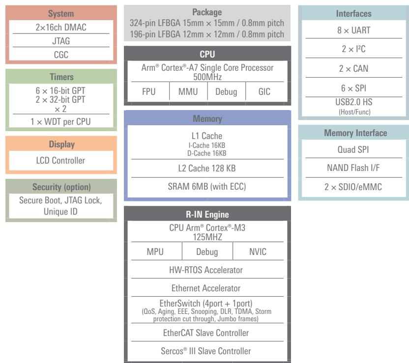
**Application example: Sensor Hub block diagram**
