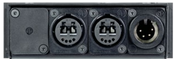
Rear view: e.g. 2R (opticalCON DUO)
