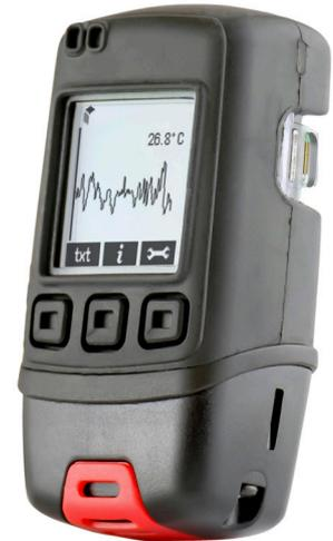
This stand-alone data logger measures and stores over 250,000 temperature readings over a -30 to +80°C (-22 to +176°F) range at a resolution of 0.1°C (0.2°F).
