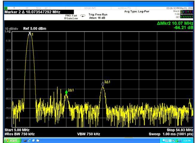
Typical direct digital synthesizer (DDS) generator has a higher noise floor and greater harmonics.
