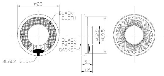
Dimensions : Millimetres Tolerance: ±0.5mm
