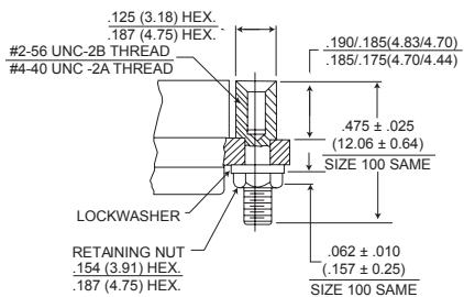
**Figure 3. Jackpost Assembly Size 9-51 Size 100\***
