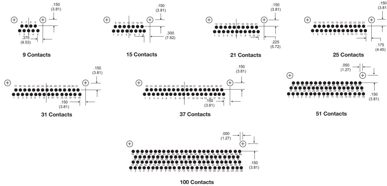
NOTE: Standard lead termination is #24 AWG, gold plated, solid copper, solder or tin dipped.
