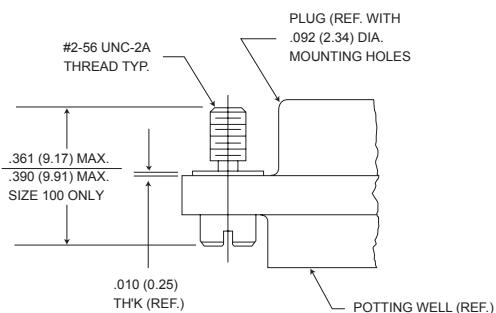
**Figure 1. Jackscrew - Low profile Slotted Head Size 9-51 Size 100\***
