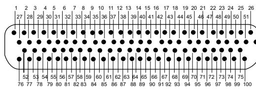
Contact identification numbers are for reference only and do not appear on insulation or connector body.
