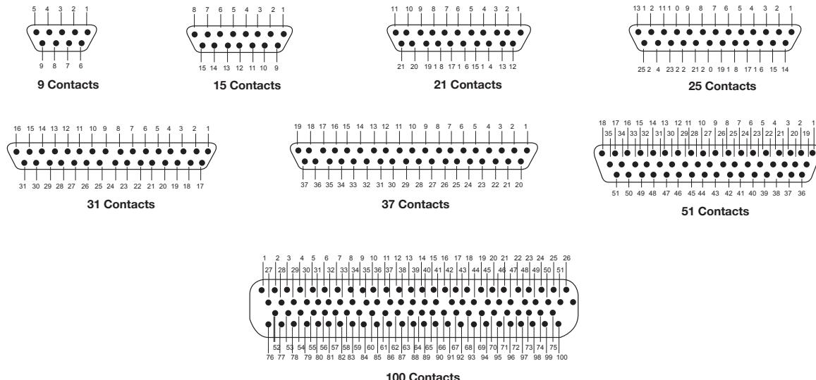
Contact identification numbers are for reference only and do not appear on insulator or connector body.
