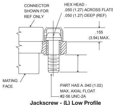
Shown here is a cutaway view of the float mount for the MDM connector. The basic shell dimensions are the same for the float mount and the screw mounting hole configurations. View shown is for standard float mount front panel mounting. Reverse mounting is available on request.
