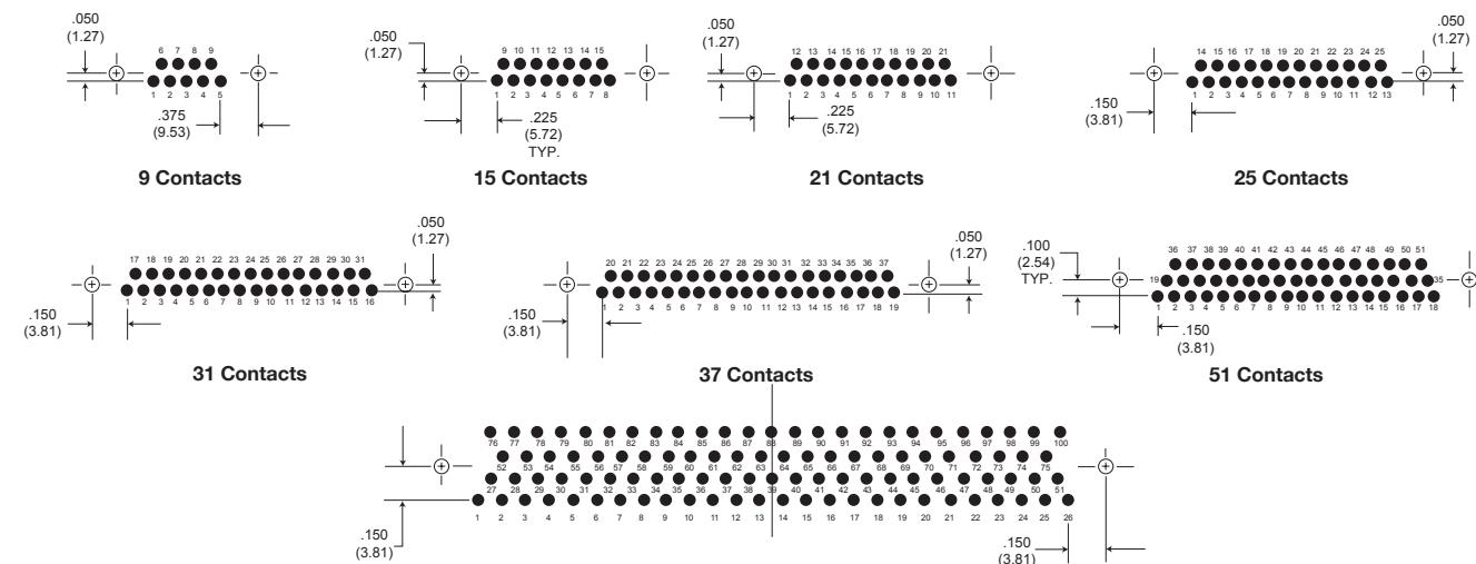
NOTE: Standard lead termination is #24 AWG, solid copper, solder or tin dipped
