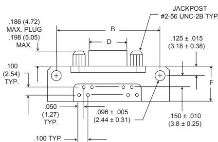
PCB Termination Arrangements (Viewed from bottom of connector, PCB solder side.)
