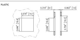
Housing: High-impact Acrylonitrile Butadiene Styrene (ABS resin), UL 94 V-0 rated
