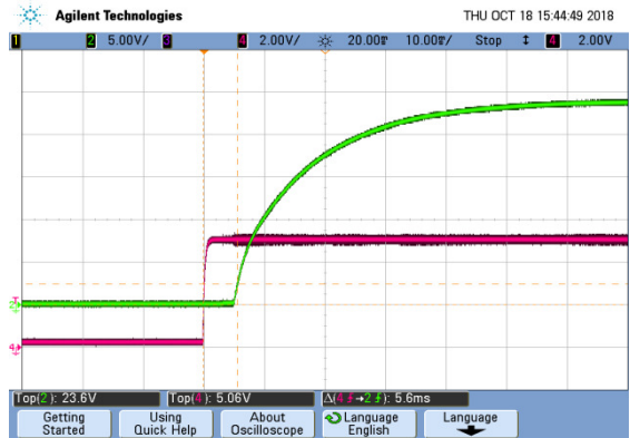
On/Off Enable Delay (Vin = 12V Vout= nom Iload =0A Load=1000μF CH2: Vout; CH4: Enable; Ta=+25°C)
