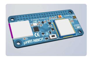
pHAT-NBIOT is a multi-band LTE Cat NB1 module that works on bands B1-5, B8, B12, B13, B17-20, B25, B28 & B66 supporting single/multitoned data and Small-Message-System (SMS) functionality. Specifically designed for the Raspberry-Pi Zero user (can also be used on all the other Raspberry-Pi variants) the pHAT-NBIOT features I<sup>2</sup>C communication to leave the Raspberry-Pi UART for other functions eg. Sensors, debug etc.
