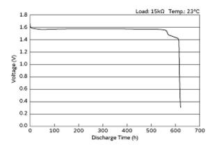
Discharge Characteristics (Load/Temperature)
