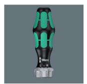
Suitable for 6 mm Wera Vario blades. Ratchet, fine-tooth design minimal for return angle, switchover ring (right, locked, left), maximum torque of up to 50 Newton metres, 6 mm hexagon chuck.<br/>
