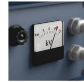
Our screwdrivers are tested for dielectric strength under a 10,000 volt load to make sure that their most important property, their insulation, has been exhaustively tested. Each individual Wera VDE screwdriver is subjected to this test to guarantee safe working up to 1,000 volts. -40°C
