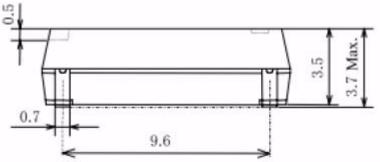
Holder Style Mode Adjustment Tolerance Temperature Stability Operating Temp. Range Load Capacitance ESR Drive Level Static Capacitance (C0) Ageing Marking CM309E Fundamental  $\pm$  50PPM at 25°C  $\pm$  100 PPM -40°C to +85°C 30 pF 150 Max Ohm 0.1 Max mW 5.0 Max pF +/-5ppm 1st Year Max Mark Std
