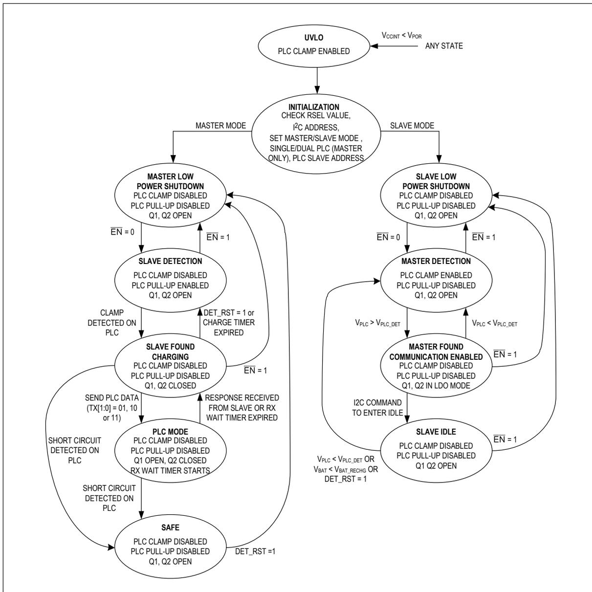
Figure 2. Master and Slave Mode Operation State Diagram
