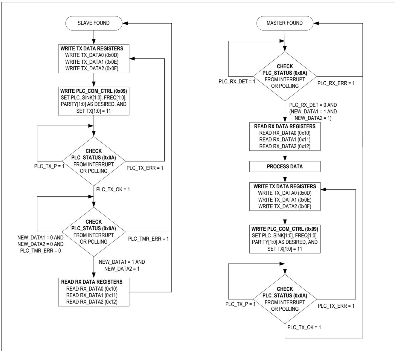
Figure 1. Flow Chart for Transmitting 3 Bytes
