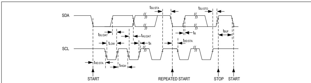
Figure 4. I<sup>2</sup>C Interface Timing
