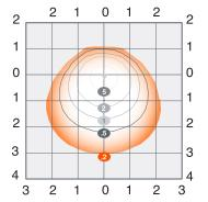
SLMFLD1A/050UNV840/WF/BZ Isofootcandle Lines at 10' Mounting Height
