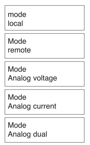
When the desired mode is displayed press the output on/off button to select it. If LOCAL or REMOTE is selected, no further setup is required and the display will return to the setup main menu.
