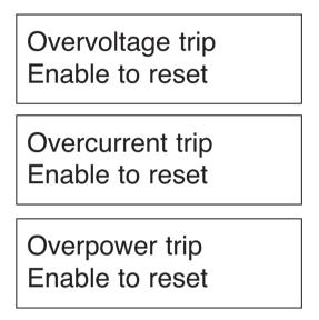
Pressing Output On/Off when any of the trip screens are displayed will reset the trip and put the power supply back in idle mode. The following screen will be displayed.
