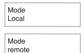
3) When REMOTE is displayed press the output on/off button. Note that when in remote mode all menu selections other than REMOTE or LOCAL are suppressed.
