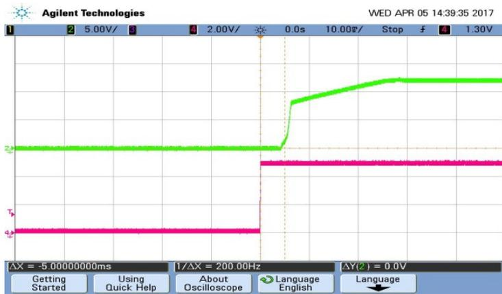
On/Off Enable Delay (Vin = 12V; Vout = nom; Load = 10A; Cload = 4700µF;
