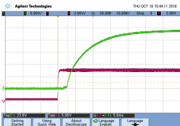
On/Off Enable Delay (Vin = 12V; Vout = nom; Load = 5A; Cloud = 1000µF;
