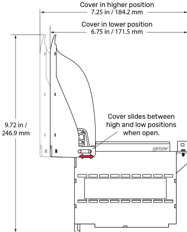
The module cover pivots and can be adjusted to two different heights (positions). The higher position provides more space to accommodate thicker wires.
