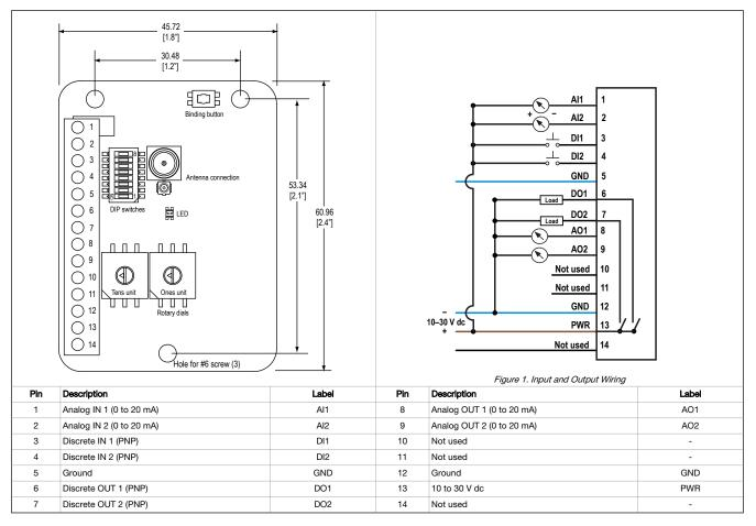
Refer to the Class I Division 2/Zone 2 control drawings (p/n 143086) for wiring specifications and limitations.
