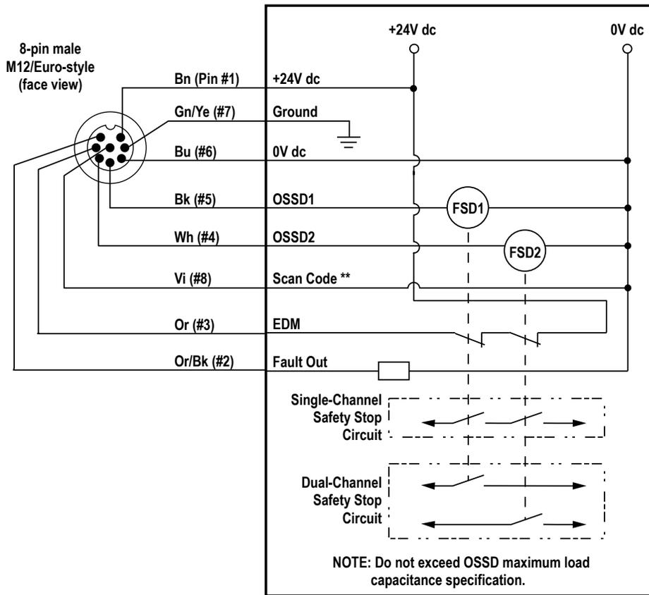
Figure 39. Generic Wiring Diagram—8-pin Receiver and Redundant FSDs
