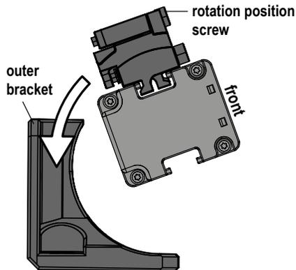
(Depending on your configuration, it may be helpful to mount the outer bracket to the mount surface first before Step 2 process)
