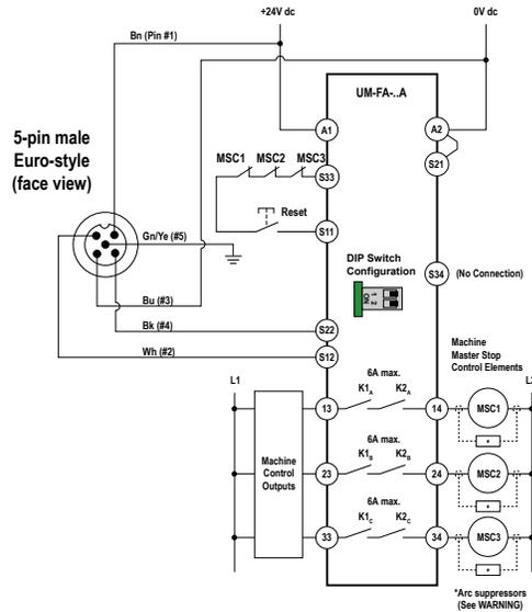
Figure 37. Generic Wiring Diagram - UM-FA..A with Manual Reset
