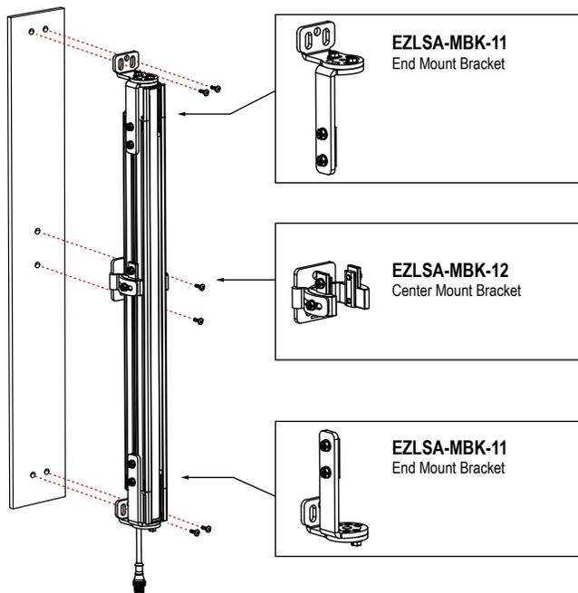
Figure 21. Mounting the center- and side-mount brackets
