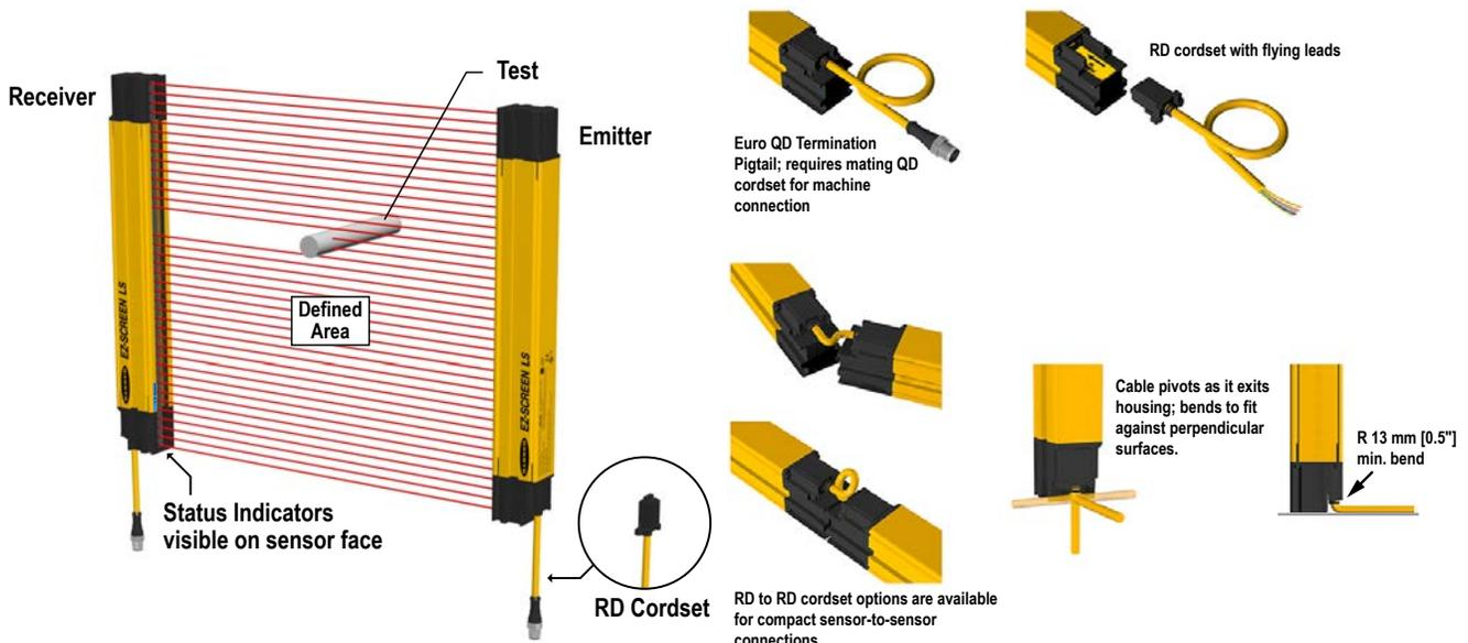
Figure 1. EZ-SCREEN LS System: Emitter, Receiver, Interconnecting Cordsets
