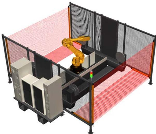
Figure 42. Light screens guarding a robotic cell
