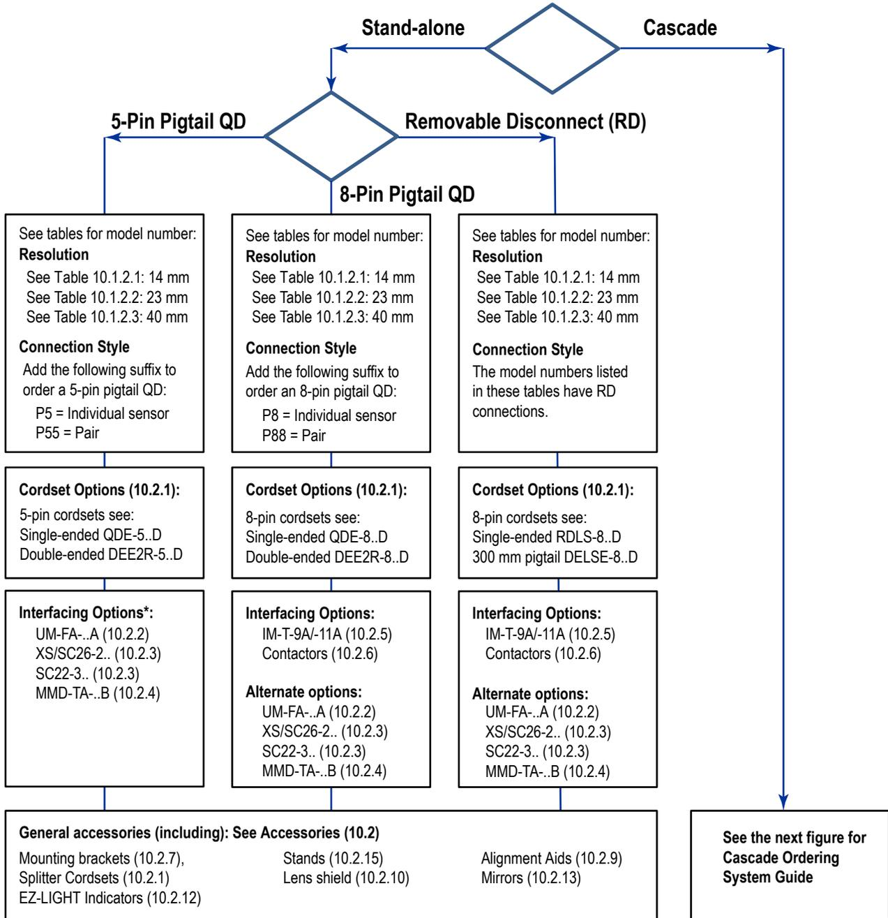
\* 5-pin models must be interfaced with a self-checking safety module, safety controller, or safety PLC/PES that conforms to the level of performance required by the risk assessment (such as Control Reliability and/or ISO13849-1 Categories 3 or 4 and PL d or e).
