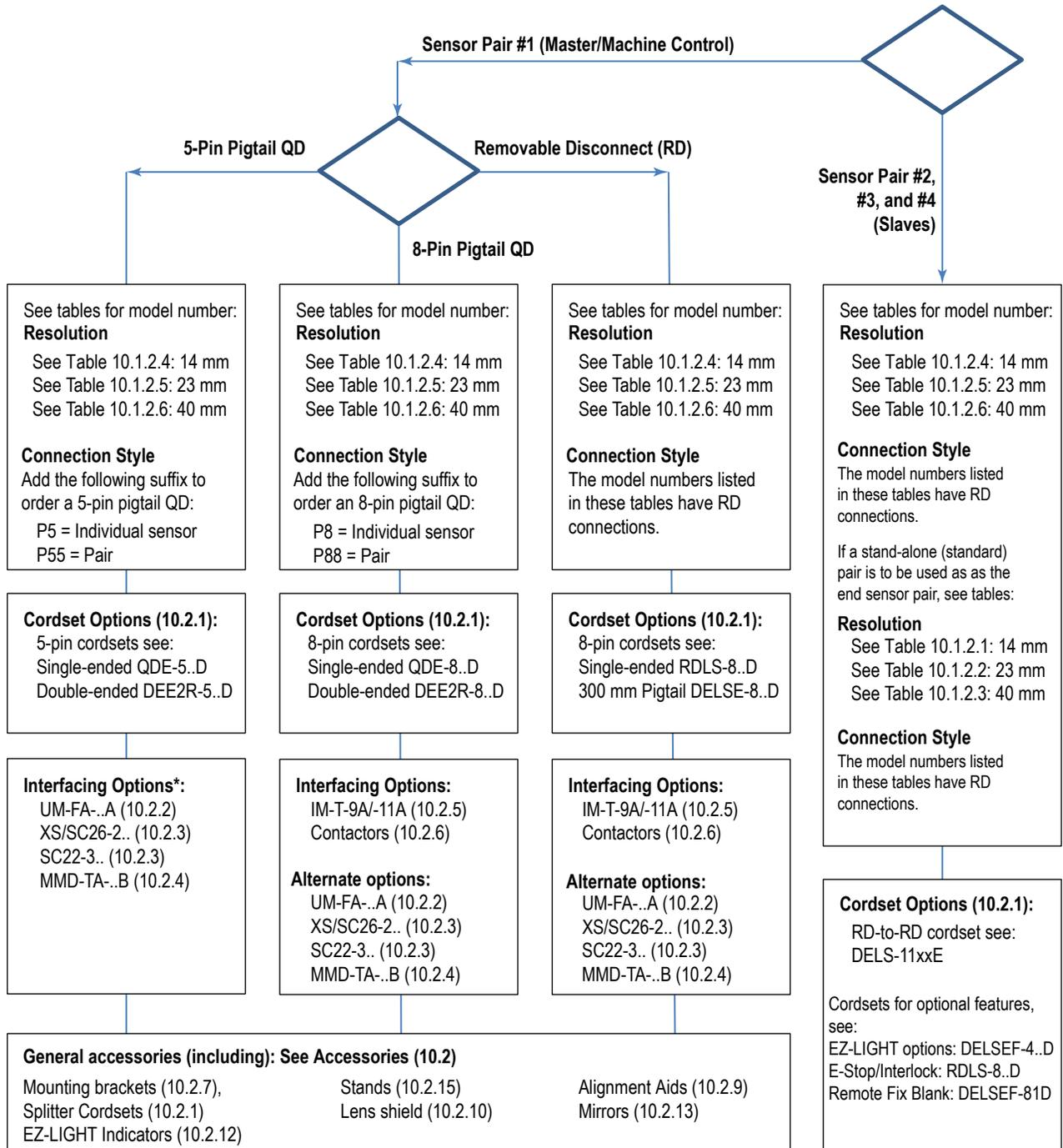
\* 5-pin models must be interfaced with a self-checking safety module, safety controller, or safety PLC/PES that conforms to the level of performance required by the risk assessment (such as Control Reliability and/or ISO13849-1 Categories 3 or 4 and PL d or e).
