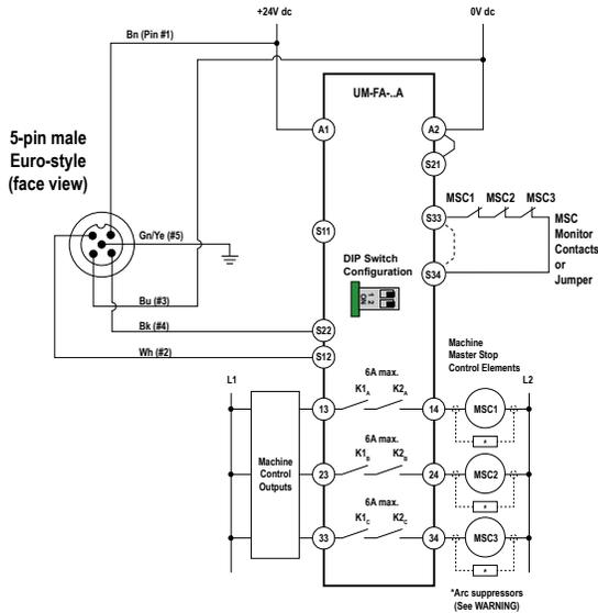
Figure 36. Generic Wiring Diagram - UM-FA..A with Auto Reset
