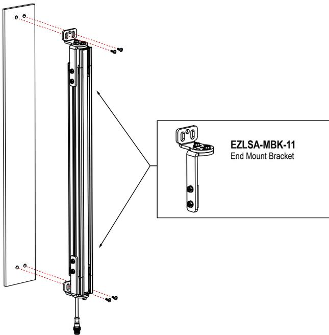
Figure 20. End-Mount Brackets
