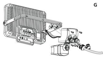
· Remove the jumper plug from the floodlight.
