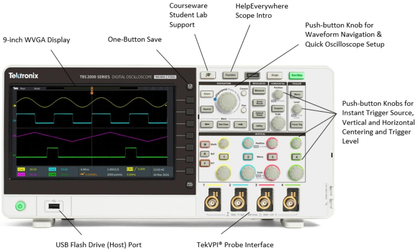
**Versatile triggering and acquisition modes** – The trigger system is designed for troubleshooting today’s mixed signal designs. Beyond a basic edge trigger, it also includes pulse width and runt triggering, which are especially useful for troubleshooting digital sections of your designs. Pulse width triggering is perfect for hunting narrow glitches or timeout conditions. Runt trigger is designed to capture signals that are shorter in amplitude than expected.
