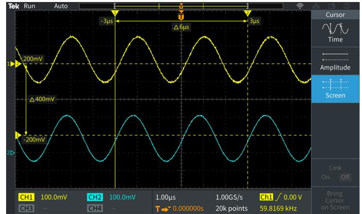
The cursor readouts are presented on the waveform display. Cursors can be used to measure time and amplitude.
