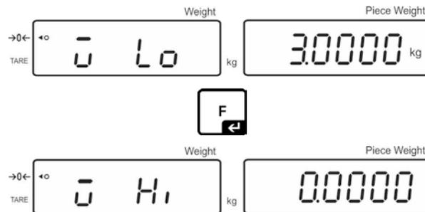
The upper limit for the target weight including current setting will be displayed.
