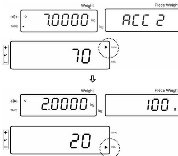
⇒ Add more weighed goods as described before. Please note that the weighing system must be unloaded between the individual weighing procedures.
