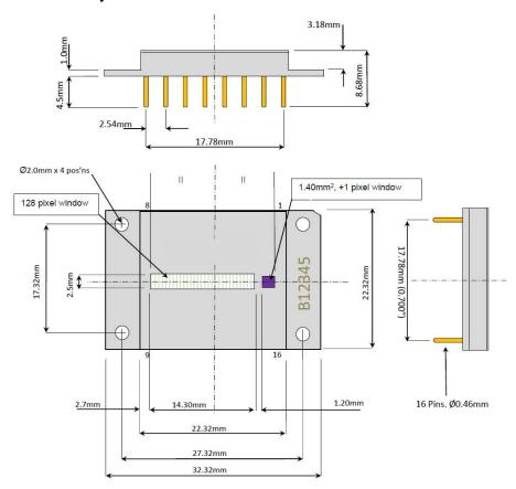
Pin Configuration of Sensor - 128+1 Element Line Sensor Array
