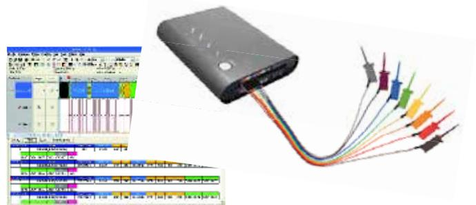
Self-contained bus-decoding probe powered via USB
