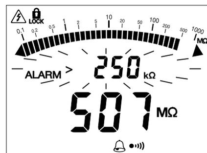
In the example above, the user can thus check that their continuity measurement is indeed less than 2 Ω, just by listening, without looking at the display unit. They can check insulation quality in the same way.
