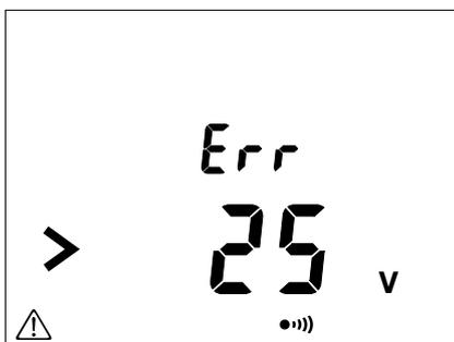
Before the insulation measurement, the instrument is in voltage measurement mode. If there is a voltage on the terminals in excess of 25 V and you try even so to make a measurement, the instrument reports the situation.
