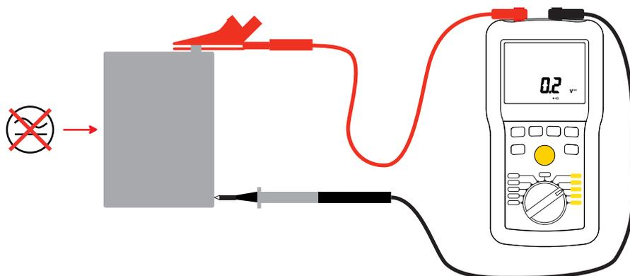
Press the **TEST** button and hold it down until the measurement displayed is stable. If a voltage greater than 25 V is detected, pressing the **TEST** button has no effect.
