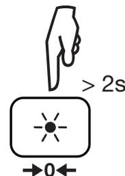
The display changes to zero and the  $\rightarrow 0 \leftarrow$  symbol is displayed. The resistance of the leads will be systematically subtracted from all continuity measurements. If the resistance of the leads is > 10  $\Omega$ , there is no compensation.
