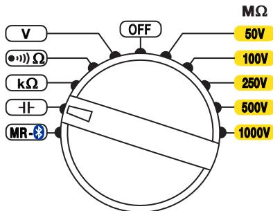
As for a continuity measurement, connect the device to be tested to the terminals of the instrument. The device to be tested must not be live (see § 2.4.3).
