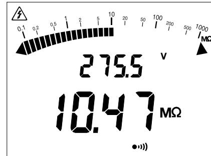
The symbol indicates that the instrument is generating a hazardous voltage (> 70 V).
