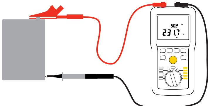
The instrument displays the voltage on the terminals. It detects whether the voltage is AC or DC and, if it is AC, displays its frequency (on the C.A 6524 and the C.A 6526).
