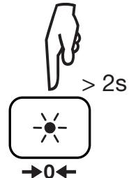
The display changes to zero and the  $\rightarrow\text{O}\leftarrow$  symbol is displayed. The resistance of the leads will be systematically subtracted from all continuity measurements. If the resistance of the leads is > 10  $\Omega$ , there is no compensation.
