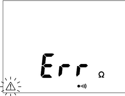
If, during a continuity, resistance, or capacitance measurement, the instrument detects an external voltage in excess of 15 V (AC or DC), it interrupts the measurement and displays the screen shown opposite.
