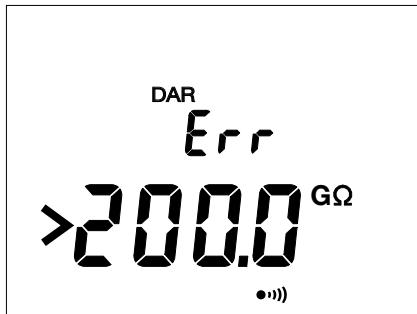
With the C.A 6524 or C.A 6526, if this occurs during a DAR or PI measurement, the instrument interrupts the measurement and displays the screen shown opposite.
