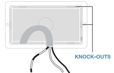
2. Select the most suitable entry point of the mounting box (knock-out) and route the supply cable through.
