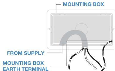
be two or three wires of each colour connected to each terminal) + an additional connection between the mounting box earth terminal and the socket earth terminal.
