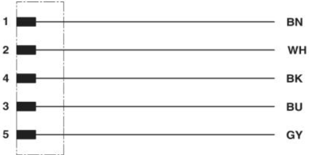
Contact assignment of the M12 connector
