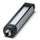
LED machine light, 24 V DC, emission angle 40 °/80 °, color temperature 5000 K, length 190 mm, diameter 40 mm, M12 connector, Light housing: Anodized aluminum, Pane: Single-pane safety glass (ESG, thermally toughened float glass), pivoting, resistant to coolants and lubricants
