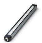
LED machine light, 24 V DC, emission angle 40  $^{\circ}$ /80  $^{\circ}$ , color temperature 5000 K, length 540 mm, diameter 40 mm, M12 connector, Light housing: Anodized aluminum, Pane: Single-pane safety glass (ESG, thermally toughened float glass), pivoting, resistant to coolants and lubricants
