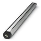
LED machine light, 24 V DC, emission angle 75 °/95 °, color temperature 5000 K, length 1070 mm, diameter 70 mm, M12 connector, Light housing: Anodized aluminum, Pane: Single-pane safety glass (ESG, thermally toughened float glass), pivoting, resistant to coolants and lubricants
