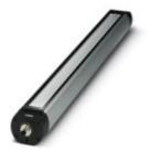
LED machine light, 24 V DC, emission angle 75 °/95 °, color temperature 5000 K, length 650 mm, diameter 70 mm, M12 connector, Light housing: Anodized aluminum, Pane: Single-pane safety glass (ESG, thermally toughened float glass), pivoting, resistant to coolants and lubricants
