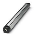
LED machine light, 24 V DC, emission angle 75 °/95 °, color temperature 5000 K, length 790 mm, diameter 70 mm, M12 connector, Light housing: Anodized aluminum, Pane: Single-pane safety glass (ESG, thermally toughened float glass), pivoting, resistant to coolants and lubricants
