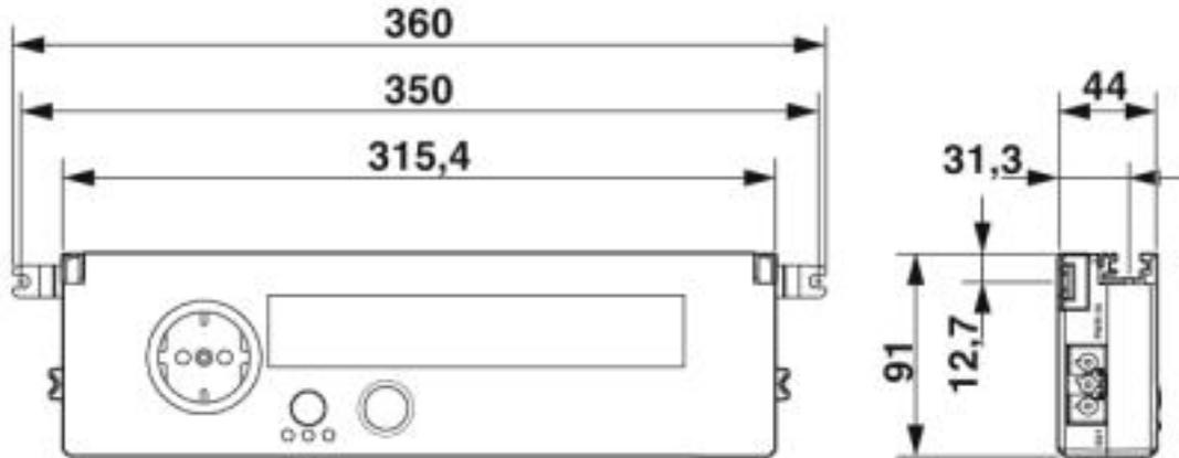
Dimensional drawing for screw mounting
