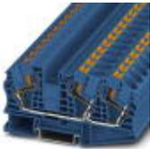
Feed-through terminal block, nom. voltage: 1000 V, nominal current: 76 A, connection method: Push-in connection, number of connections: 3, cross section: 0.5 mm<sup>2</sup> - 25 mm<sup>2</sup>, AWG: 20 - 4, width: 12.2 mm, height: 53.3 mm, color: blue, mounting type: NS 35/7,5, NS 35/15
