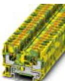
Ground modular terminal block, connection method: Push-in connection, number of connections: 2, cross section: 0.5 mm<sup>2</sup> - 10 mm<sup>2</sup>, AWG: 20 - 8, width: 8.2 mm, height: 42.2 mm, color: green-yellow, mounting type: NS 35/7,5, NS 35/15
