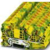
Ground modular terminal block, connection method: Push-in connection, number of connections: 3, cross section: 0.5 mm<sup>2</sup> - 25 mm<sup>2</sup>, AWG: 20 - 4, width: 12.2 mm, height: 53.3 mm, color: green-yellow, mounting type: NS 35/7,5, NS 35/15
