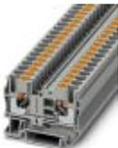
Feed-through terminal block, nom. voltage: 1000 V, nominal current: 41 A, connection method: Push-in connection, number of connections: 2, cross section: 0.5 mm<sup>2</sup> - 10 mm<sup>2</sup>, AWG: 20 - 8, width: 8.2 mm, height: 42.2 mm, color: gray, mounting type: NS 35/7,5, NS 35/15
