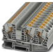
Feed-through terminal block, nom. voltage: 1000 V, nominal current: 76 A, connection method: Push-in connection, number of connections: 3, cross section: 0.5 mm<sup>2</sup> - 25 mm<sup>2</sup>, AWG: 20 - 4, width: 12.2 mm, height: 53.3 mm, color: gray, mounting type: NS 35/7,5, NS 35/15
