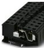
Spring-cage terminal block-fuse terminal block for cartridge fuse inserts with screw cap, cross section: 0.5 - 6 mm<sup>2</sup>, width: 12 mm, color: black
