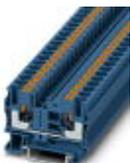
Feed-through terminal block, nom. voltage: 1000 V, nominal current: 41 A, connection method: Push-in connection, number of connections: 2, cross section: 0.5 mm<sup>2</sup> - 10 mm<sup>2</sup>, AWG: 20 - 8, width: 8.2 mm, height: 42.2 mm, color: blue, mounting type: NS 35/7,5, NS 35/15
