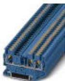
Feed-through terminal block, nom. voltage: 800 V, nominal current: 24 A, connection method: Push-in connection, number of connections: 3, cross section: 0.14 mm<sup>2</sup> - 4 mm<sup>2</sup>, AWG: 26 - 12, width: 5.2 mm, height: 35.2 mm, color: blue, mounting type: NS 35/7,5, NS 35/15
