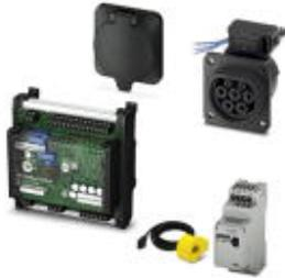
HOME charging technology set starter kit for easy assembly of a charging station, Integrated release function of the locking actuator for disconnection of Infrastructure Plug and Infrastructure Socket Outlet, IEC 62196-2, IEC 61851-1, Mode 3, Case B, 11 kW, 16 A, 400 V AC, cable: 0.7 m
