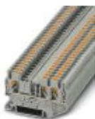
Feed-through terminal block, nom. voltage: 800 V, nominal current: 24 A, connection method: Push-in connection, number of connections: 3, cross section: 0.14 mm<sup>2</sup> - 4 mm<sup>2</sup>, AWG: 26 - 12, width: 5.2 mm, height: 35.2 mm, color: gray, mounting type: NS 35/7,5, NS 35/15
