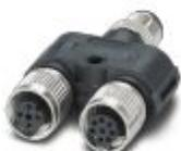
Y distributor for PSR-CT series RFID transponder switches, M12 male/female, 5- and 8-pos., for signal contact feedback to the PLC
