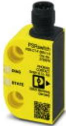
Proximity safety circuit up to Cat. 4, PL e (EN ISO 13849), SIL 3 (IEC 61508), multicode sensor with RFID coding, model 4 (EN ISO 14119), automatic or manual start, integrated diagnostics, 24 V DC supply, IP69K, M12 connector
