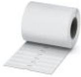
Marking foil for zack marker strip, Roll, white, unlabeled, can be labeled with: THERMOMARK ROLL 2.0, THERMOMARK ROLL, THERMOMARK ROLL X1, THERMOMARK ROLLMASTER 300/600, THERMOMARK X1.2, mounting type: adhesive, for terminal block width: 104 mm, lettering field size: 104 x 10 mm, Number of individual labels: 1500
