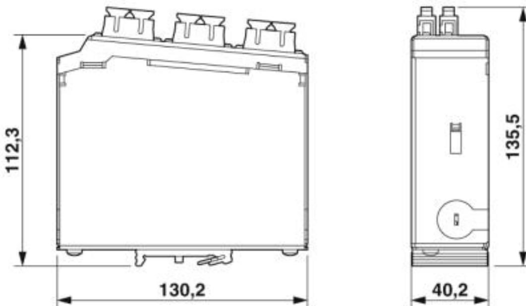
DIN rail splice box 6x SC duplex OS2, fully mounted ready to splice
