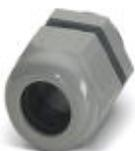
Cable gland, cable gland material: PA, external cable diameter 6 mm ... 12 mm, shielding: no, connecting thread: M20 x 1.5, color: silver-gray RAL 7001
