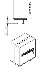
Pin 2 and 3 are only for mechanical stability.
