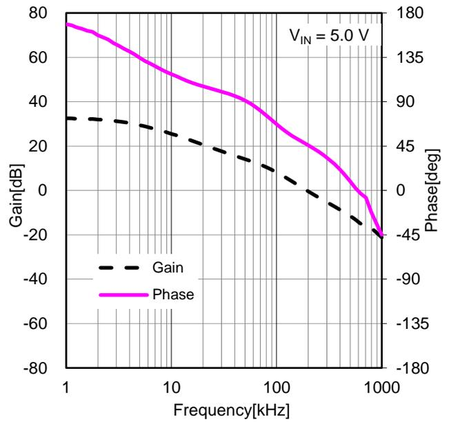
Figure 32. Frequency Characteristics ( $I_{OUT} = 2\text{ A}$ )
