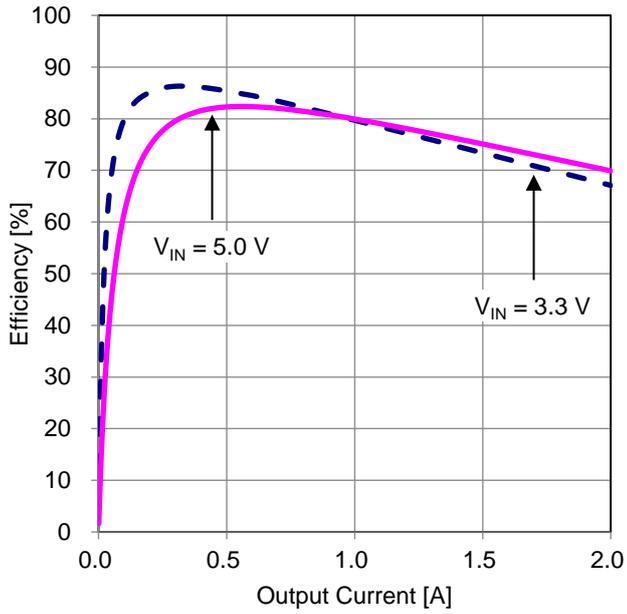
Figure 31. Efficiency vs Output Current
