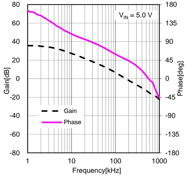
Figure 37. Frequency Characteristics ( $I_{OUT} = 2\text{ A}$ )
