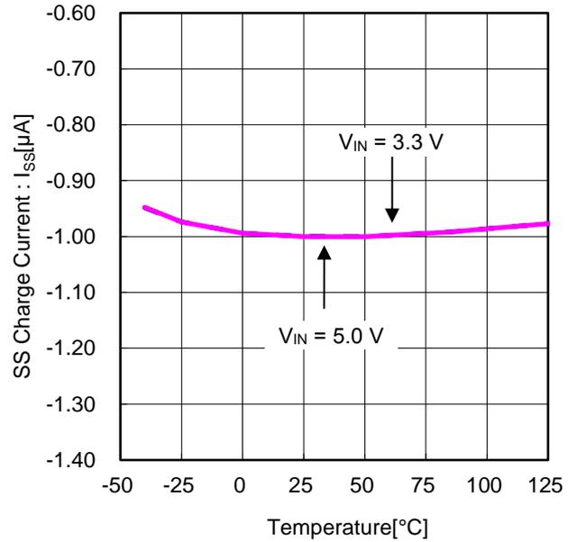
Figure 8. SS Charge Current vs Temperature
