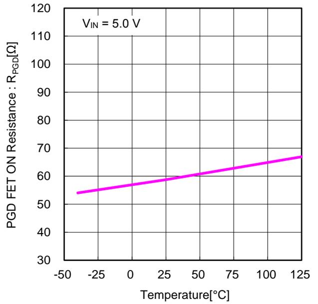
Figure 12. PGD FET ON Resistance vs Temperature
