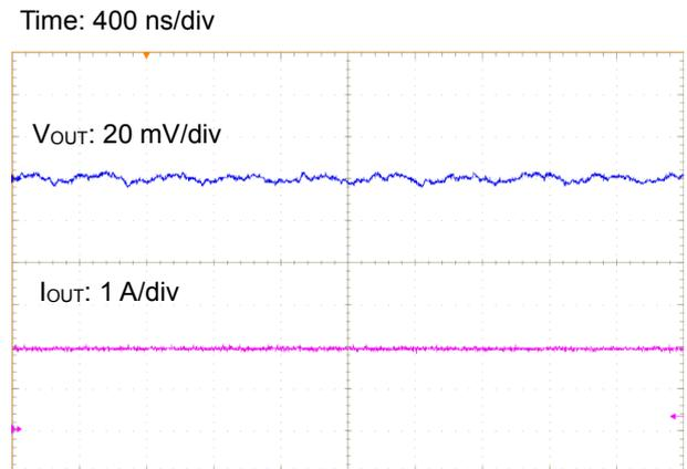
Figure 44. Output Ripple Voltage ( $I_{OUT} = 2\text{ A}$ )
