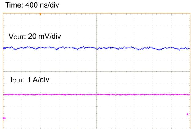
Figure 34. Output Ripple Voltage ( $I_{OUT} = 2\text{ A}$ )
