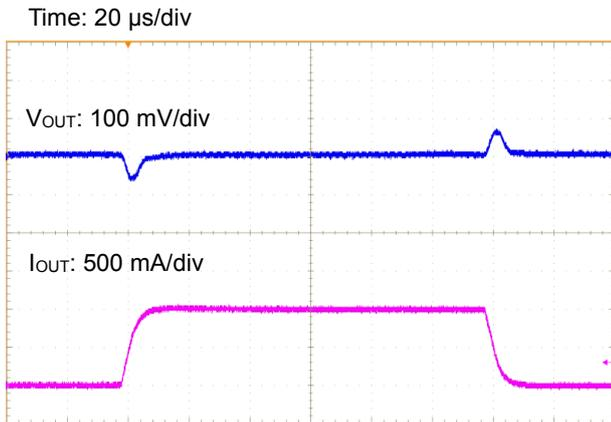
Figure 38. Load Transient Response ( $I_{OUT} = 0\text{ A} \leftrightarrow 1\text{ A}$ )
