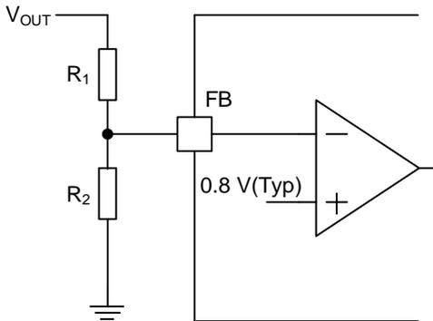
$$V_{OUT} = \frac{R_1 + R_2}{R_2} \times 0.8 \text{ [V]}$$
