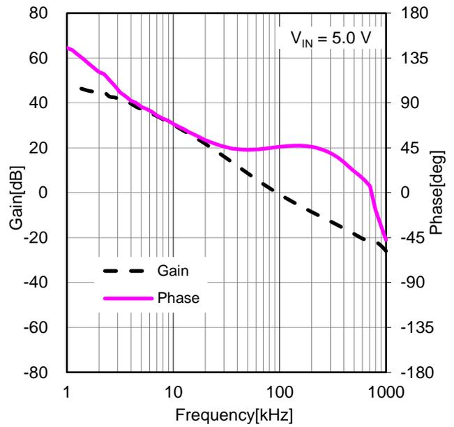
Figure 52. Frequency Characteristics ( $I_{OUT} = 2\text{ A}$ )
