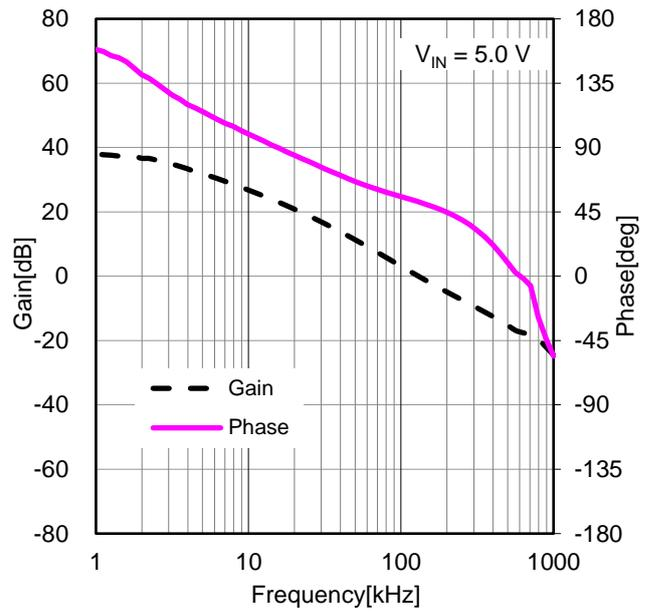
Figure 47. Frequency Characteristics ( $I_{OUT} = 2\text{ A}$ )
