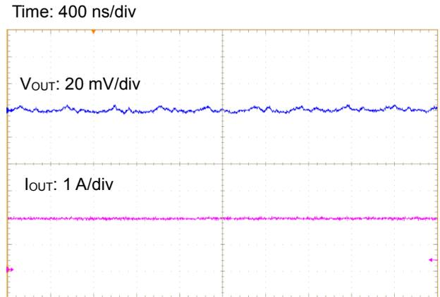
Figure 54. Output Ripple Voltage ( $I_{OUT} = 2\text{ A}$ )
