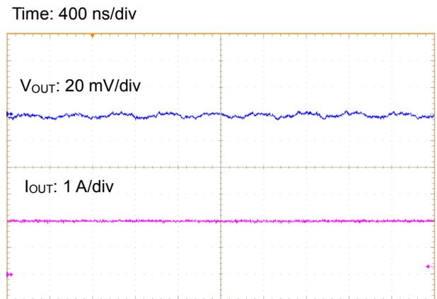
Figure 49. Output Ripple Voltage ( $I_{OUT} = 2\text{ A}$ )
