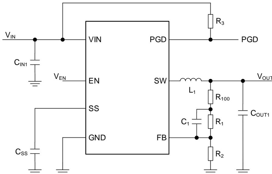
Figure 35. Reference Circuit 2
