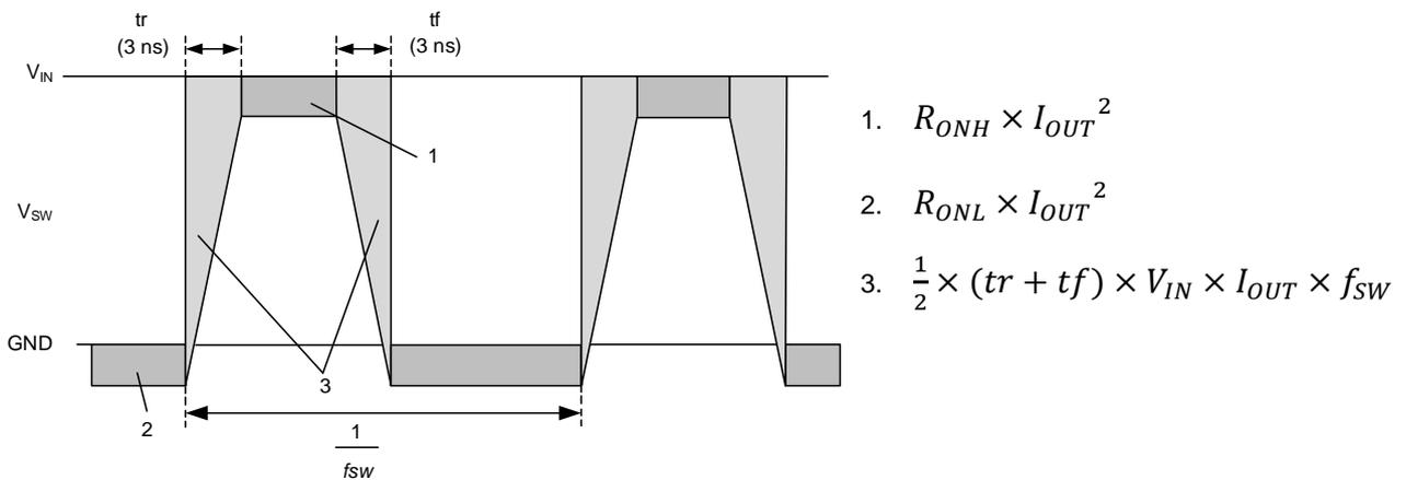
Figure 59. SW Waveform
