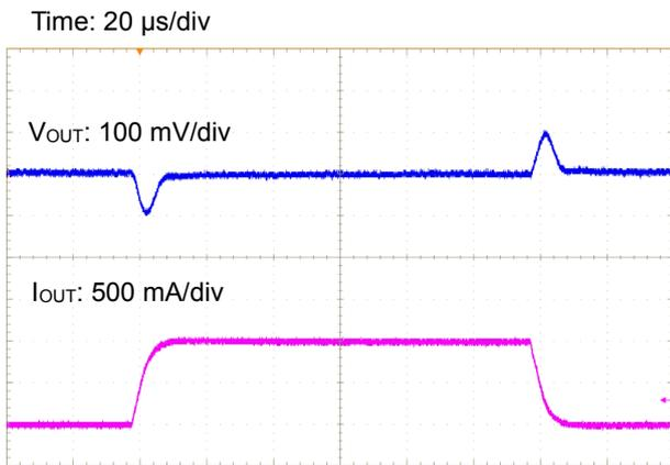
Figure 48. Load Transient Response ( $I_{OUT} = 0\text{ A} \leftrightarrow 1\text{ A}$ )
