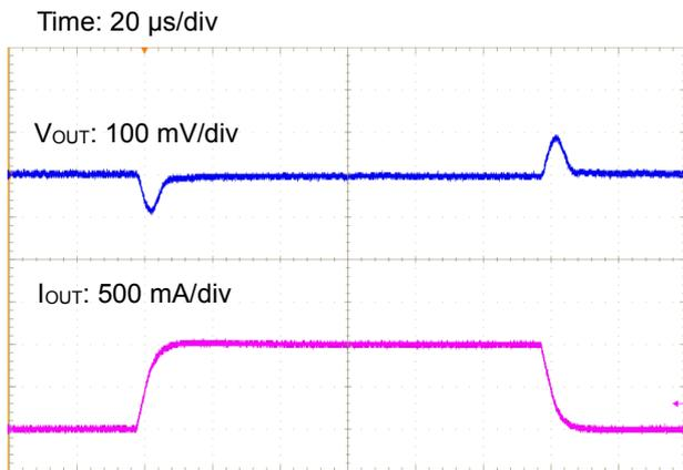
Figure 43. Load Transient Response ( $I_{OUT} = 0\text{ A} \leftrightarrow 1\text{ A}$ )
