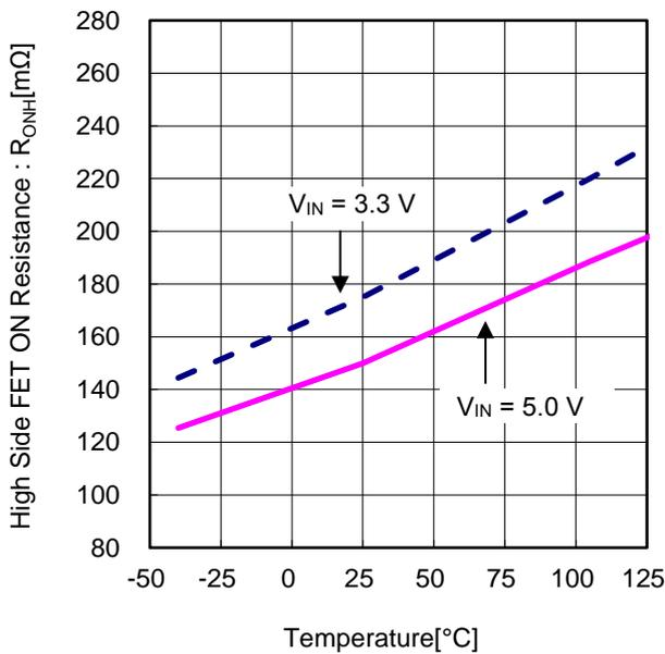
Figure 9. High Side FET ON Resistance vs Temperature
