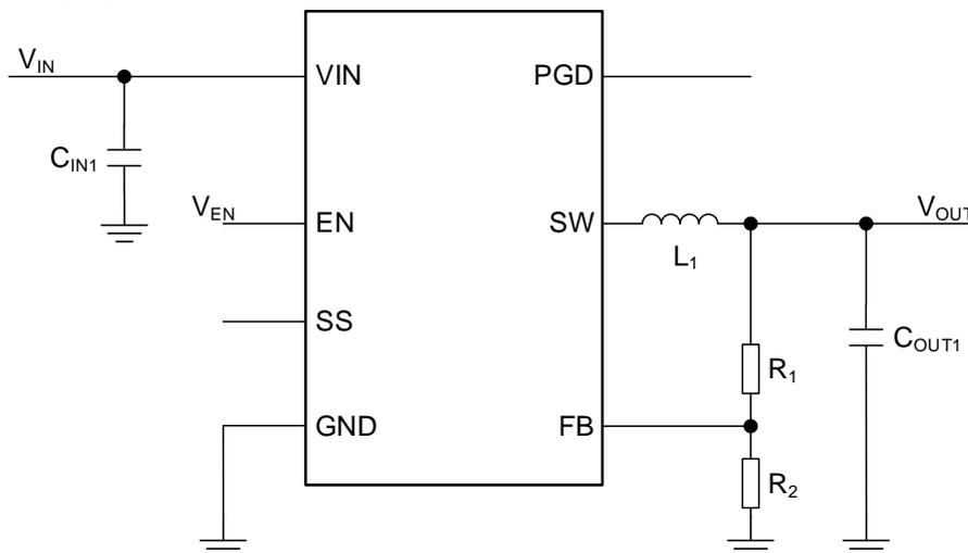
Figure 1. Application Circuit
