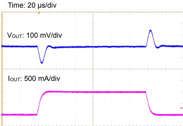
Figure 53. Load Transient Response ( $I_{OUT} = 0\text{ A} \leftrightarrow 1\text{ A}$ )
