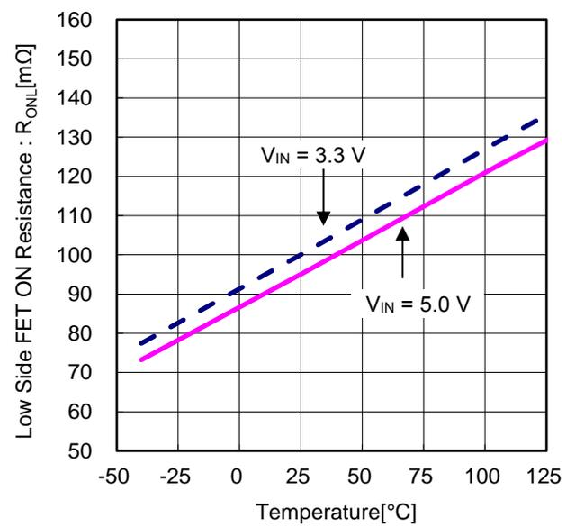
Figure 10. Low Side FET ON Resistance vs Temperature
