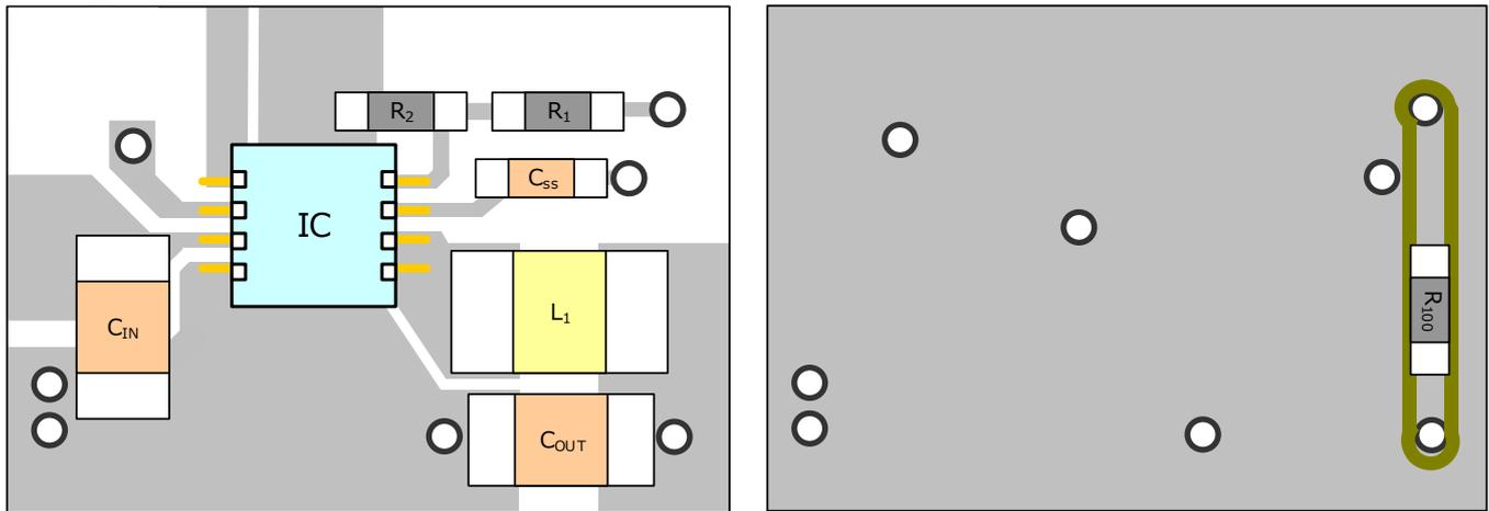
Example of Evaluation Board Layout (Top View)
