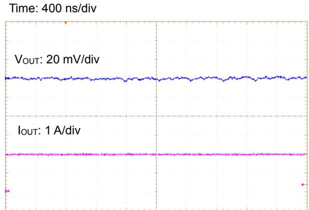
Figure 39. Output Ripple Voltage ( $I_{OUT} = 2\text{ A}$ )
