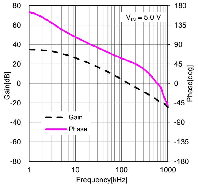
Figure 42. Frequency Characteristics ( $I_{OUT} = 2\text{ A}$ )
