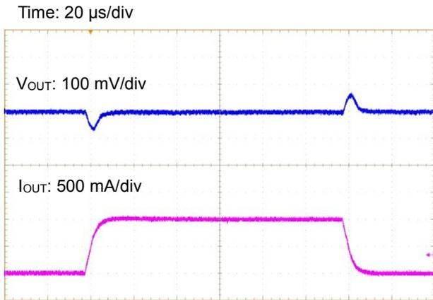
Figure 33. Load Transient Response ( $I_{OUT} = 0\text{ A} \leftrightarrow 1\text{ A}$ )
