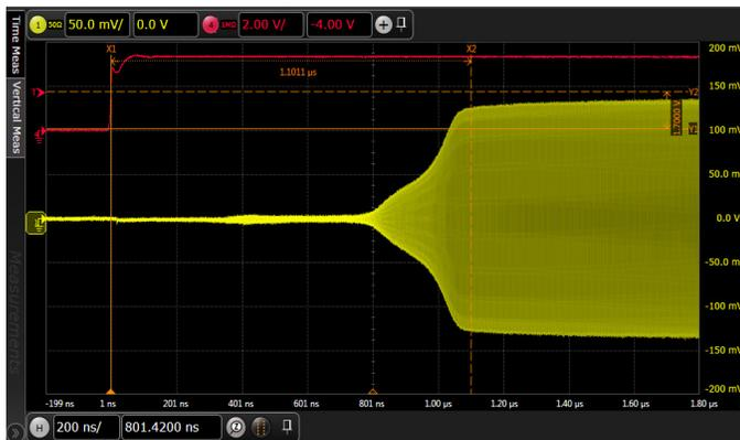
Figure 25. Switching Time [Insertion Loss to Isolation State]
